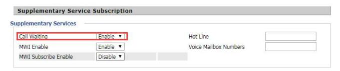
Step 3. At position 1, you can configure whether to enable the call waiting function.
