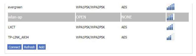
Step 4. If the connected wireless does not have a password, you can connect directly; if the wireless connection has a password, enter the password and click "OK" to confirm the connection.
